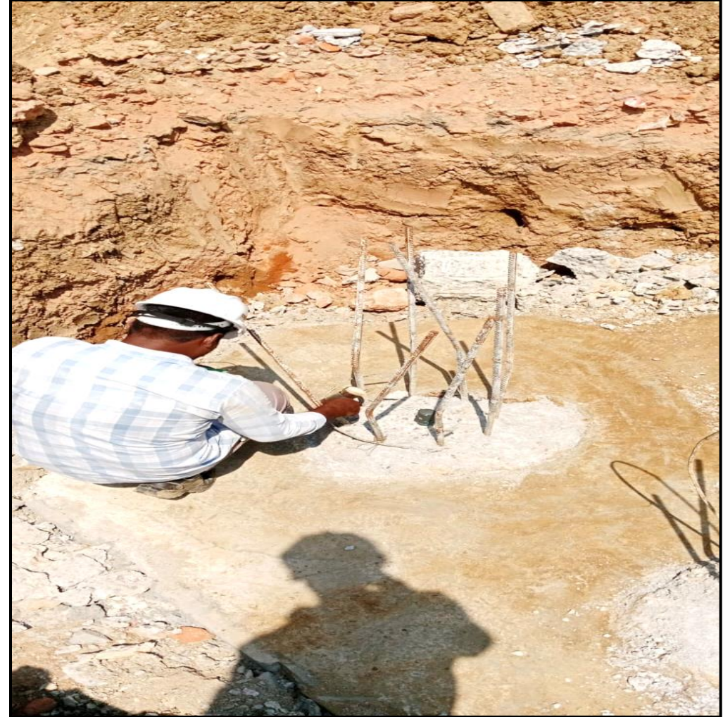
Pile integrity test work in progress (77/220 Nos completed)
