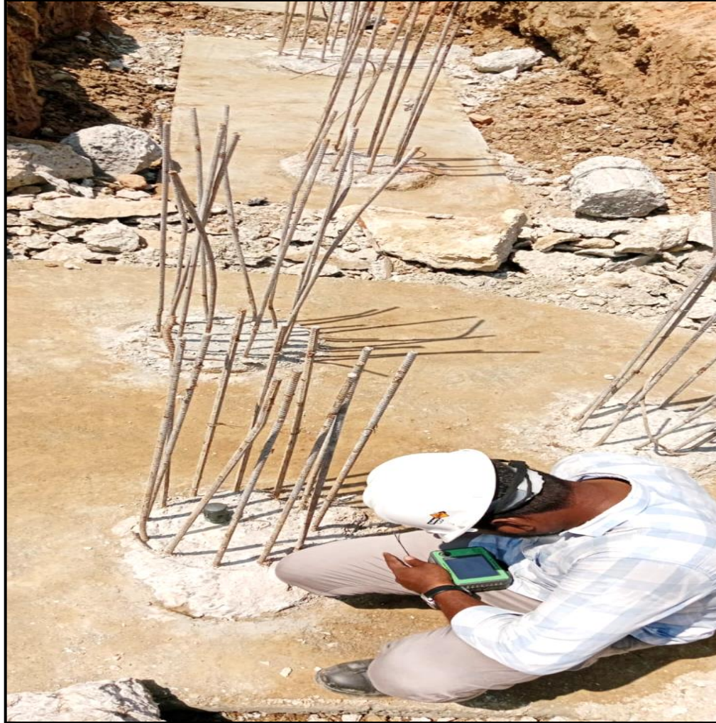
Pile integrity test work in progress (77/220 Nos completed)
