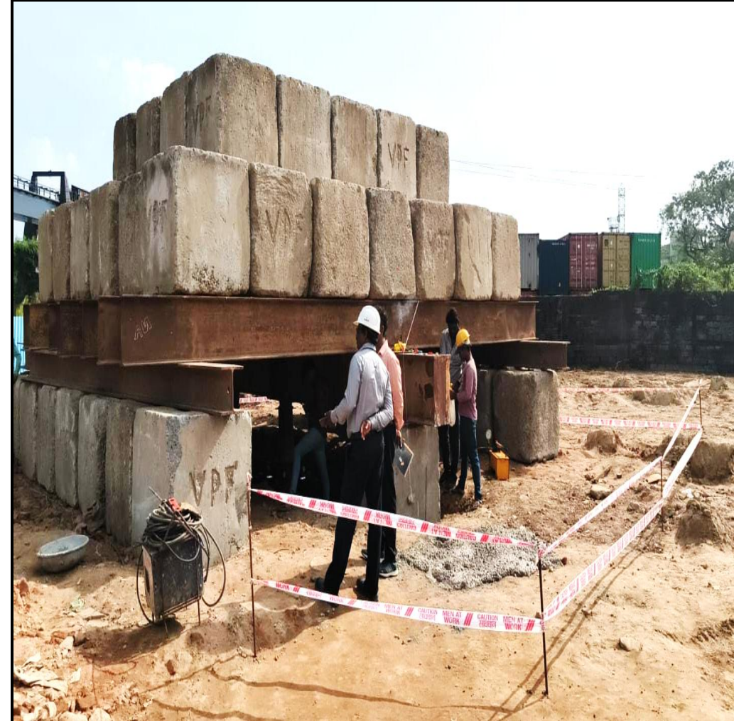
Static load test work completed- Pile No 60
