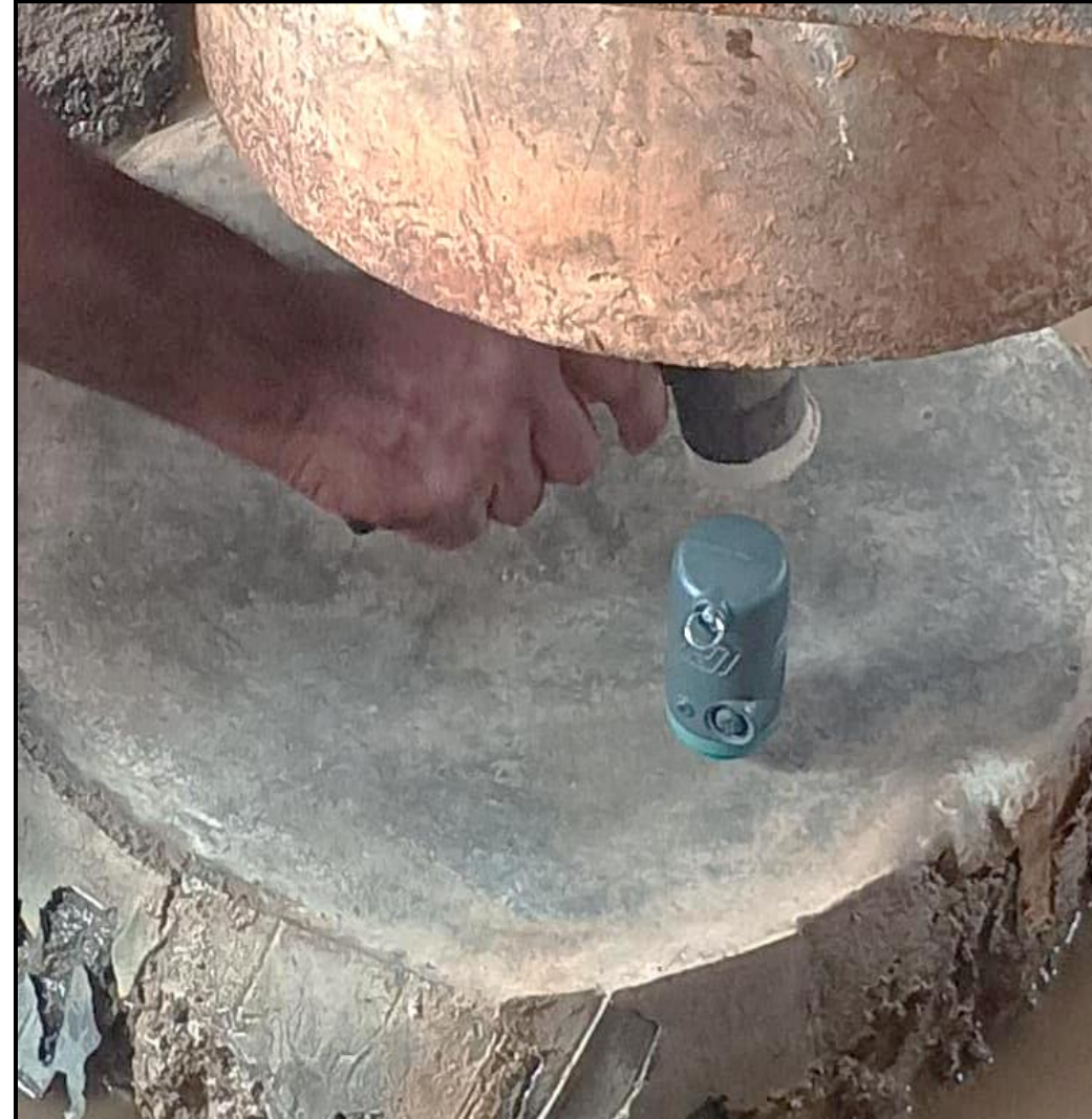
Pile integrity test 2 no's completed
