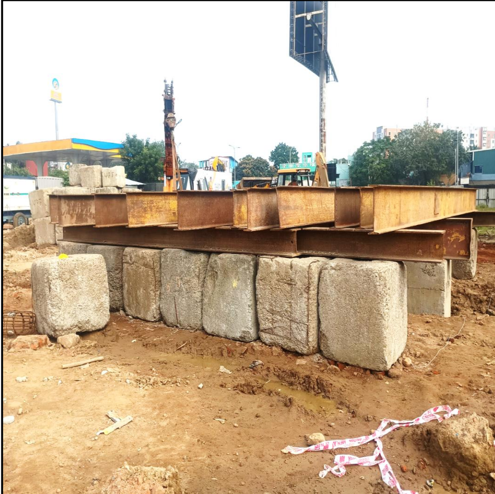
Static load test work completed- Pile No 60
