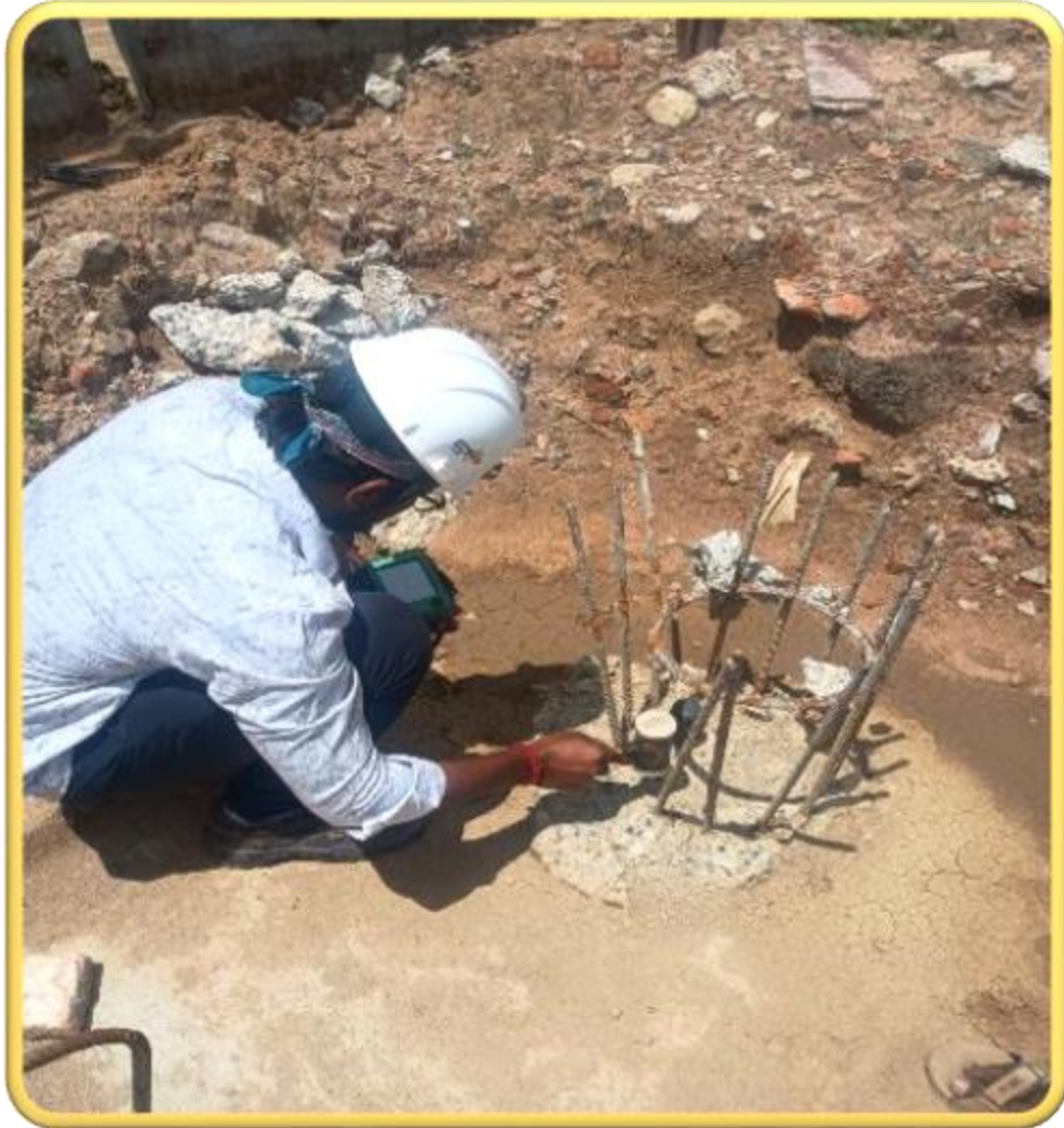
Amenity building – Pile Integrity Test
