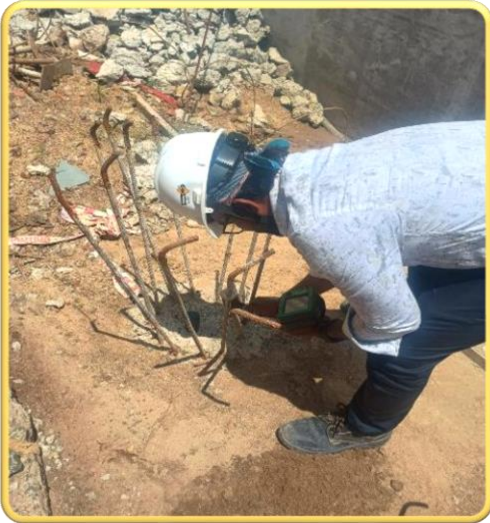
Amenity building – Pile Integrity Test
